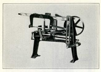
Atkins Kwik-Kut Machine, Nos. 14 and 12 (Push -Cutting)
