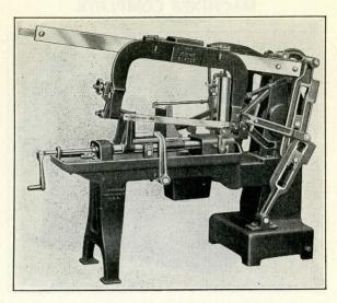
Atkins Kwik-Kut Machine No. 7, a Draw Cut Machine
