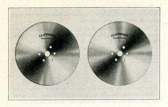
Friction Discs are used at the mills and in structural shops for cutting off rails, steel bars, and structural shapes. Sometimes they are used with a plain edge, but better results can be secured with an upset or nicked edge, because these discs pass through the metal by creating heat with friction, and the nicked edge secures a better contact with the metal.
